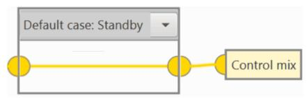
• **Flight Control Check**: In this flight phase, the Control mix variable has value **1.0** since it is necessary for the aircraft to act in FW configuration.
